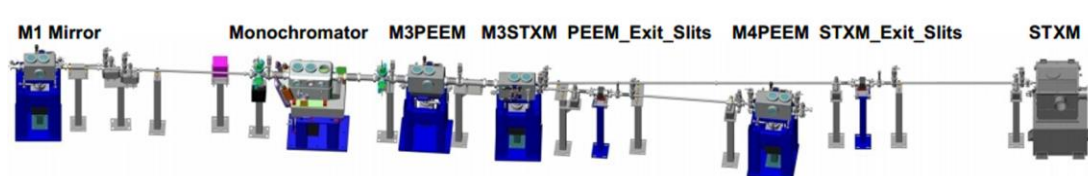
Figure 2-5 Layout of SM beamlines at CLS (courtesy of Canadian Light Source Inc.) [10].
